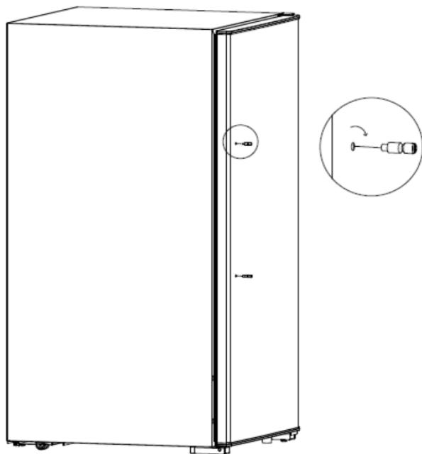
2. There are two holes on the handle base, fix the handle screws into the handle base hole as below:
