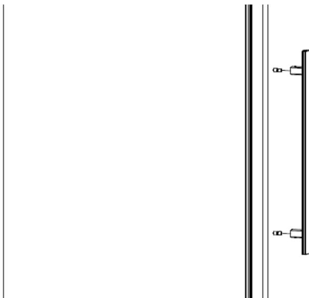
3. After handle is fixed onto the handle screw on the door, there are two hexagon screws popping out, use a hexagon screw driver to fix the screws as below:
